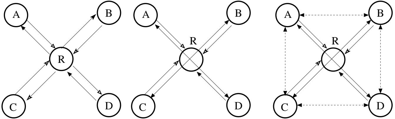
Specifically, the cases are (a) pure relaying, where packets are not combined, (b) network coding, where two packets are combined, and (c) network coding with overhearing, where the relay combines four packets.
